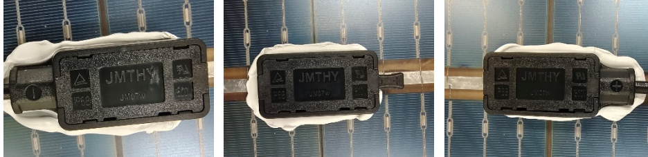
Fig. 3: View of junction box of module type ERA Pro-72HCB585M
